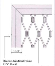
Emtek #103 Amplimesh (1/4" thick extrusion)
